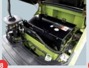
Easy Access to the Battery The bonnet can be opened wide to check the battery and facilitate access to the truck interior.
