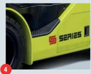
Large Metal Step The driver enters the ergonomically designed interior via a large, low, non-slip step.
