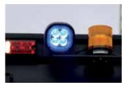
**Blue LED Warning Lights** The blue LED warning lights provide a visual warning for both directions of travel.
